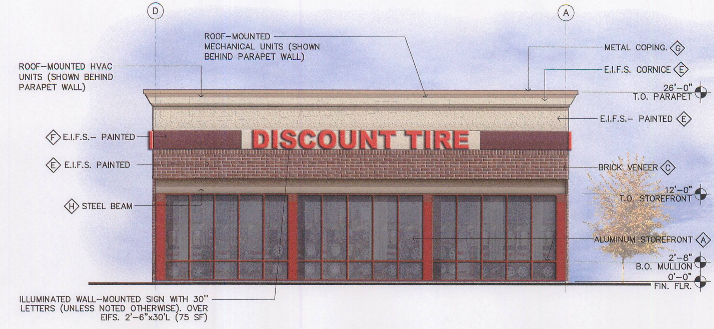
EAST ELEVATION (E. Independence Blvd) SCALE: 1/8" = 1'-0"
