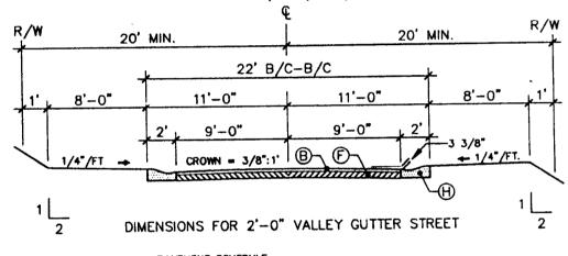
1 1/2" BITUMINOUS CONCRETE SURFACE COURSE, TYPE I-2
