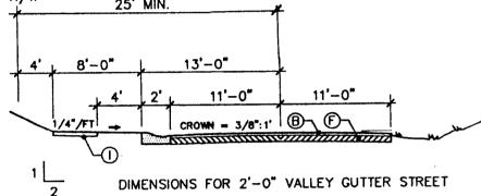
PAVEMENT SCHEDULE (B) 1 1/2" BITUMINOUS CONCRETE SURFACE COURSE, TYPE 1-2
