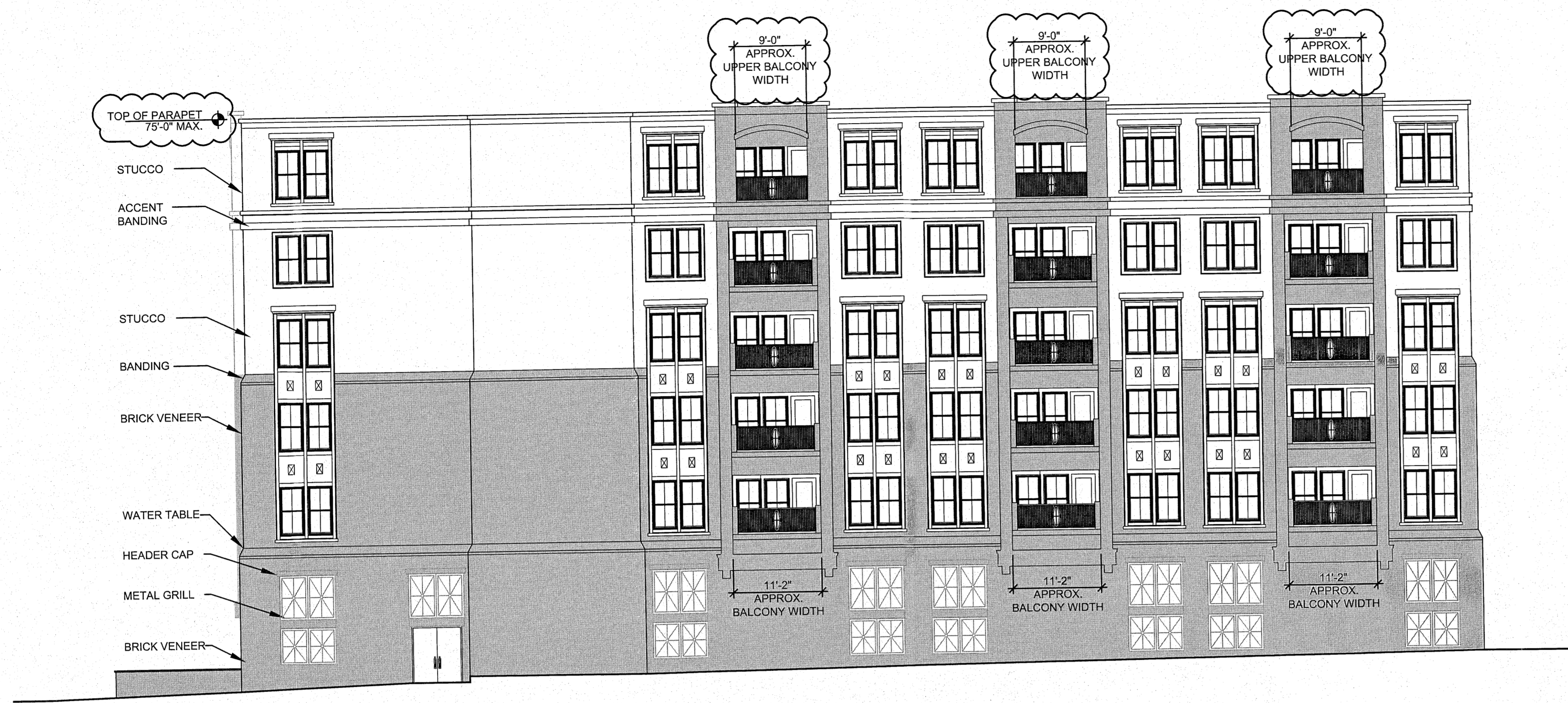
4 BUILDING 1 - SOUTH ELEVATION SCALE: 3/32" = 1'-0"
