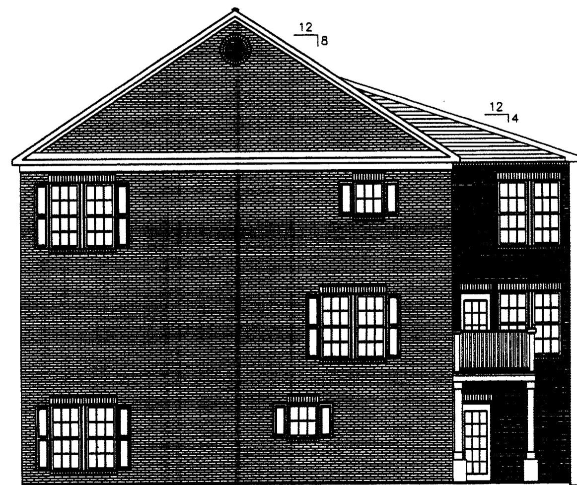
13 FRONT LOADED SIDE ELEVATION @ CHURCH / WINNIFRED A-6 SCALE: 1/8" = 1'-0" (WITH OPTIONAL THREE-STORY SUNROOM) (NOTE: THIS ELEVATION ONLY WHERE THE BUILDING SIDE OF FRONT LOADED UNITS ABUT CHURCH OR WINNIFRED STREETS)
