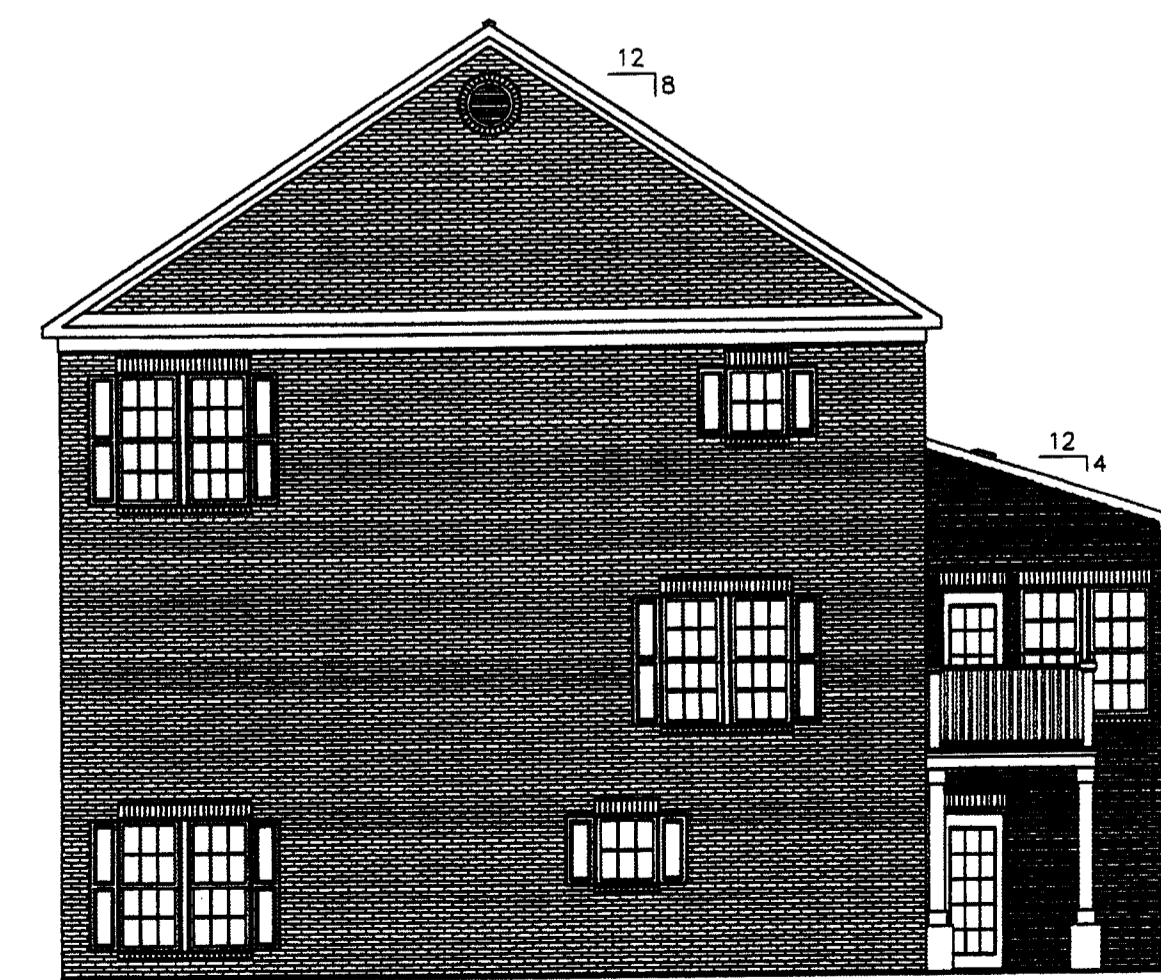
11 FRONT LOADED SIDE ELEVATION @ CHURCH / WINNIFRED A-6 SCALE: 1/8" = 1'-0" (WITH OPTIONAL TWO-STORY SUNROOM) (NOTE: THIS ELEVATION ONLY WHERE THE BUILDING SIDE OF FRONT LOADED UNITS ABUT CHURCH OR WINNIFRED STREETS)
