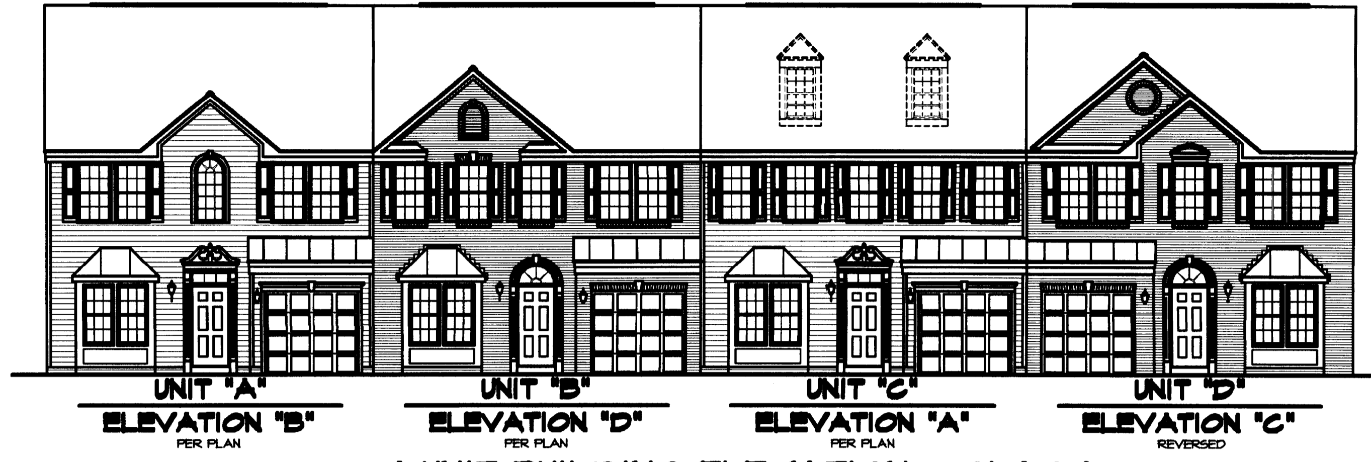
1 A-1 4 UNIT BUILDING ELEVATION - GLA04 SCALE: 1/8" = 1'-0"
