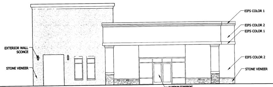
**04** MALLARD CREEK CHURCH RD. EXTERIOR ELEVATION
