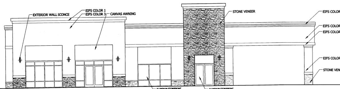
**02** ACCESS DRIVE EXTERIOR ELEVATION
