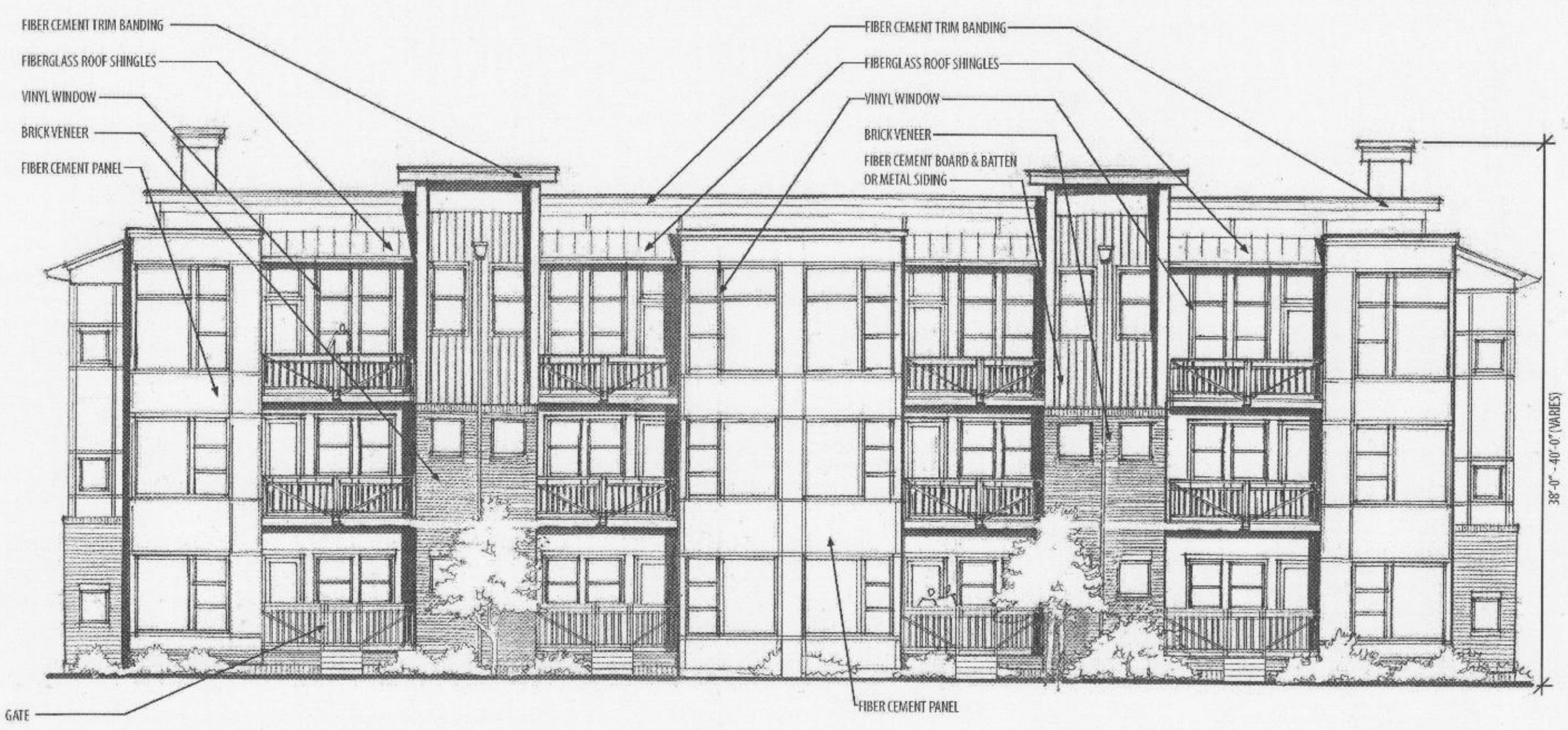
TYPICAL PARKWOOD STREET FRONT BUILDING ELEVATION
