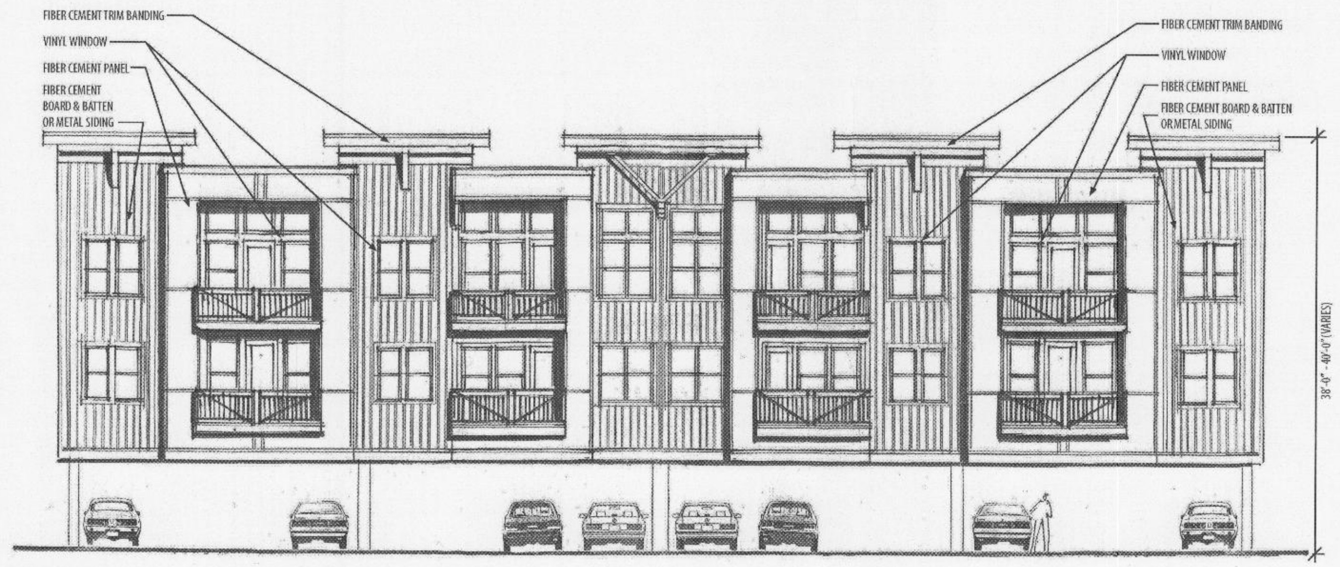
TYPICAL PARKWOOD REAR BUILDING ELEVATION
