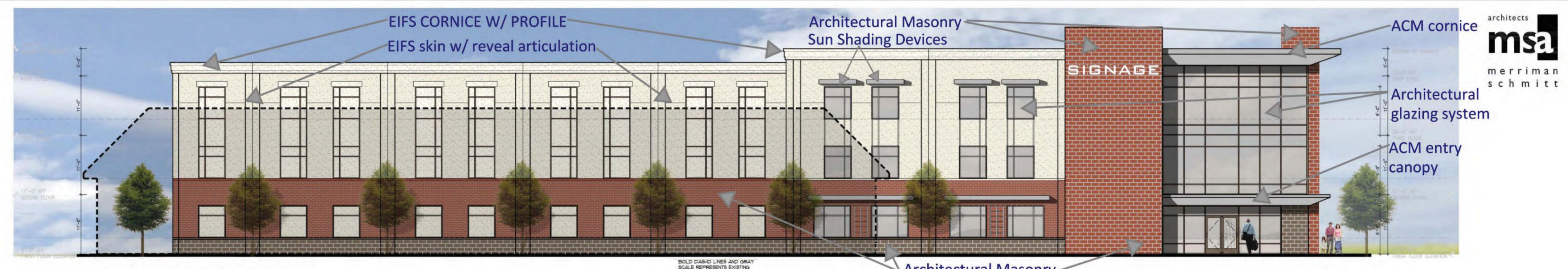
Building 2 - EAST ELEVATION
