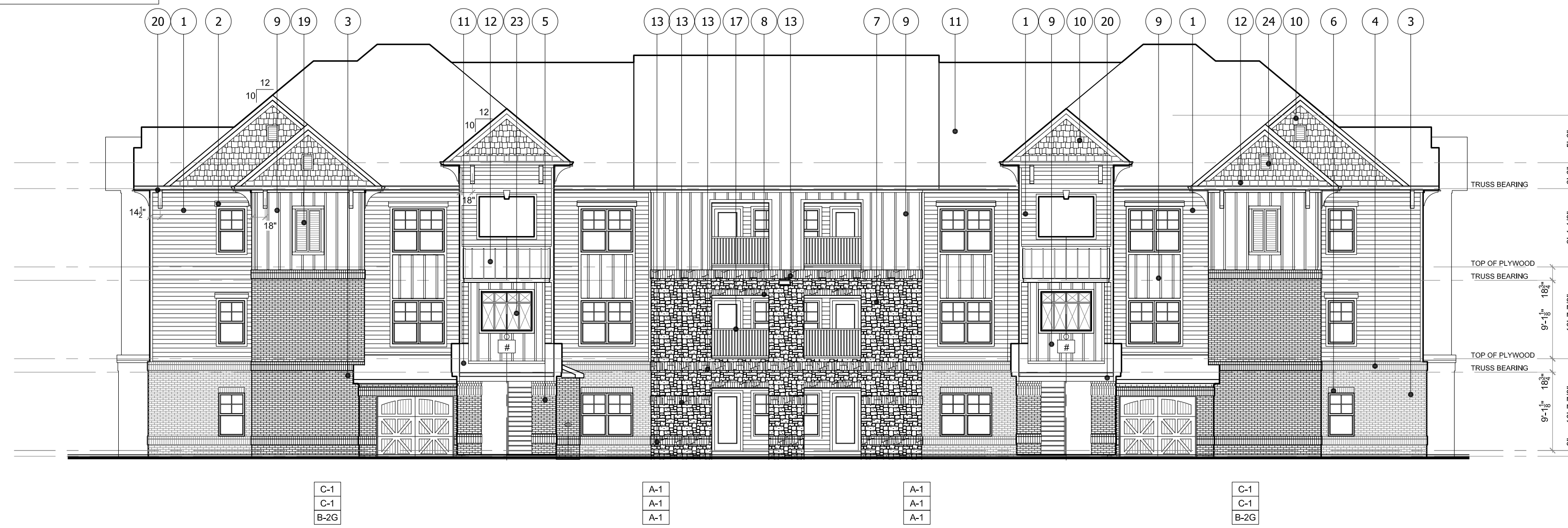
1 TYPE 3 (BLDG - 1) - FRONT ELEVATION
