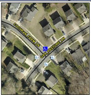
Street 1 Name Stop Condition-Street 2 Street 2 Name Stop Condition-Street 1 **COCHRAN FARM LN** StopSign **OAK PASTURE LN** None Possible Solutions: Remove & Replace Curb Ramp With Two New Directional Ramps or Equivalent. Surveyor Notes: N/A PROW/ADA: Not Found, R304.5.1, R304.2.2, R304.5.3
