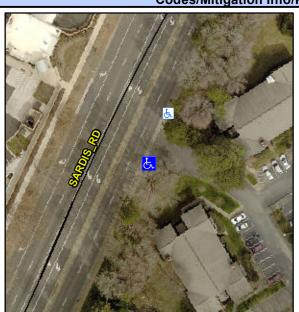
**ENTRANCE** Street 1 Name Stop Condition-Street 2 None Street 2 Name **SARDIS RD** Stop Condition-Street 1 None Possible Solutions: Remove & Replace Curb Ramp With **Two New Directional Ramps or** Equivalent. Surveyor Notes: N/A PROW/ADA: Not Found, R304.2.2, R304.5.3
