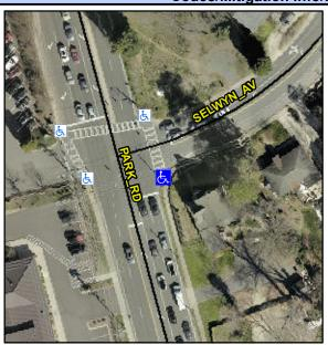
**SELWYN AV** Street 1 Name Stop Condition-Street 2 Signal **PARK RD** Street 2 Name Stop Condition-Street 1 Signal Possible Solutions: Remove & Replace Curb Ramp With Two New Directional Ramps or Equivalent. Surveyor Notes: N/A PROW/ADA: R304.2.2
