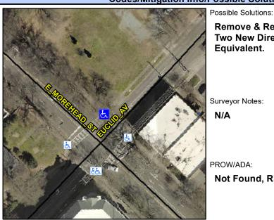
Stop Condition-Street 2 Street 2 Name Stop Condition-Street 1 Remove & Replace Curb Ramp With Two New Directional Ramps or Equivalent.
