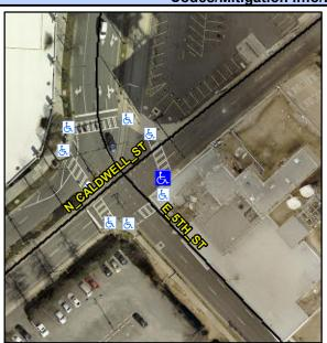
E 5TH ST Street 1 Name Stop Condition-Street 1 Signal Street 2 Name N/A Stop Condition-Street 2 N/A Possible Solutions: Remove & Replace Curb Slope and Extend Ramp. Restripe Crosswalk. Relocate Obstruction. Surveyor Notes: N/A PROW/ADA: Not Found, R207.1, R302.3, R402.2
