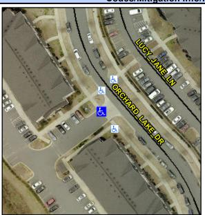
**ENTRANCE** Street 1 Name Stop Condition-Street 1 StopSign Street 2 Name N/A Stop Condition-Street 2 N/A Possible Solutions: Remove & Replace Curb Ramp With Two New Directional Ramps or Equivalent. Surveyor Notes: N/A PROW/ADA: R304.5.3
