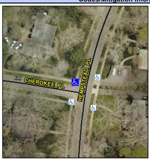
**CHEROKEE PL** Street 1 Name Stop Condition-Street 2 StopSign **HEMPSTEAD PL** Street 2 Name Stop Condition-Street 1 None Possible Solutions: Remove & Replace Curb Ramp With Two New Directional Ramps or Equivalent. Surveyor Notes: N/A PROW/ADA: Not Found, R304.5.1, R304.2.2, R304.5.3
