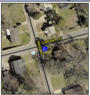
**CARONIA ST** Street 1 Name Stop Condition-Street 2 StopSign Street 2 Name **REID AV** Stop Condition-Street 1 None Possible Solutions: Remove & Replace Curb Ramp With Two New Directional Ramps or Equivalent. Surveyor Notes: N/A PROW/ADA: Not Found, R304.5.1, R304.5.3
