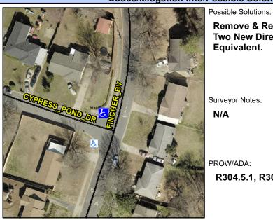
**CYPRESS POND DR** Street 1 Name Stop Condition-Street 1 StopSign Street 2 Name N/A Stop Condition-Street 2 N/A Remove & Replace Curb Ramp With Two New Directional Ramps or Equivalent.
