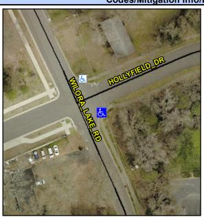
**HOLLYFIELD DR** Street 1 Name Stop Condition-Street 1 StopSign N/A Street 2 Name Stop Condition-Street 2 N/A Possible Solutions: Remove & Replace Curb Ramp With Two New Directional Ramps or Equivalent. Surveyor Notes: N/A PROW/ADA: Not Found, R304.5.1
