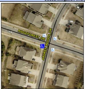
Street 1 Name Stop Condition-Street 2 Street 2 Name Stop Condition-Street 1 ARDREY WOODS DR None RIDGEFOREST DR StopSign Possible Solutions: **Remove & Replace Curb Ramp With** Two New Directional Ramps or Equivalent. Surveyor Notes: N/A PROW/ADA: Not Found, R304.5.1, R304.2.2, R304.5.3
