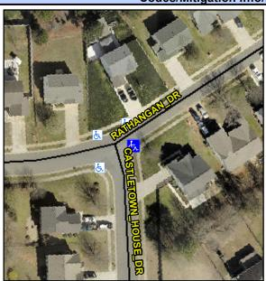
Stree Stop Stree Stop Possible Solutions: Remove & Replace Curb Ramp With Two New Directional Ramps or Equivalent.
