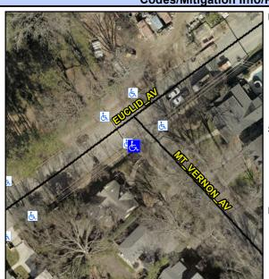
MT VERNON AV Street 1 Name Stop Condition-Street 1 StopSign Street 2 Name N/A Stop Condition-Street 2 N/A Possible Solutions: Remove & Replace Entire Ramp. Surveyor Notes: N/A PROW/ADA: R304.5.1, R304.2.2, R304.5.3
