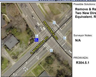
Remove & Replace Curb Ramp With Two New Directional Ramps or Equivalent. Restripe Crosswalk.
