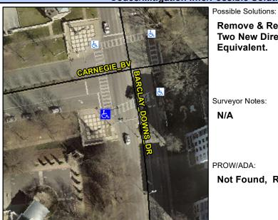
**BARCLAY DOWNS DR** Street 1 Name Stop Condition-Street 2 Signal Street 2 Name **CARNEGIE BV** Stop Condition-Street 1 Signal Remove & Replace Curb Ramp With **Two New Directional Ramps or** Equivalent.
