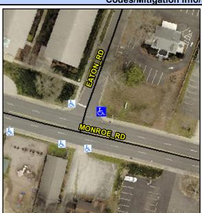
**EATON RD** Street 1 Name Stop Condition-Street 2 StopSign MONROE RD Street 2 Name Stop Condition-Street 1 None Possible Solutions: Remove & Replace Curb Ramp With Two New Directional Ramps or Equivalent. Surveyor Notes: N/A PROW/ADA: Not Found, R304.2.2, R304.5.3
