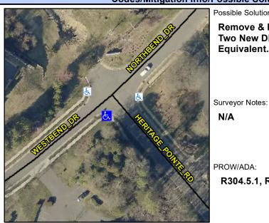
Street 1 Name Stop Condition-Street 2 Street 2 Name Stop Condition-Street 1 HERITAGE POINTE DR None **WESTBEND DR** StopSign Possible Solutions: **Remove & Replace Curb Ramp With** Two New Directional Ramps or Equivalent.
