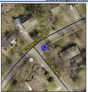
Street 1 Name Stop Condition-Street 2 Street 2 Name Stop Condition-Street 1 **CHERRYCREST LN** None **ASHCREST DR** StopSign Possible Solutions: **Remove & Replace Curb Ramp With Two New Directional Ramps or** Equivalent. Surveyor Notes: N/A PROW/ADA: Not Found, R304.2.2, R304.5.3
