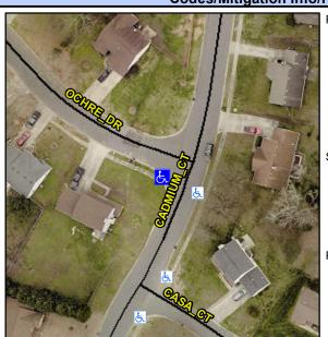
**CADMIUM CT** Street 1 Name Stop Condition-Street 1 None Street 2 Name N/A Stop Condition-Street 2 N/A Possible Solutions: Remove & Replace Entire Ramp. Surveyor Notes: N/A PROW/ADA: R304.5.1, R304.2.2
