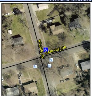
**CARLYLE DR** Street 1 Name Stop Condition-Street 2 StopSign Street 2 Name N/A Stop Condition-Street 1 N/A Possible Solutions: Remove & Replace Entire Ramp. Remove & Replace Gutter. Surveyor Notes: N/A PROW/ADA: Not Found, R304.2.1, R304.2.2-Perp, R304.3.2-Para, R305.2, R302.7.2, R304.5.4
