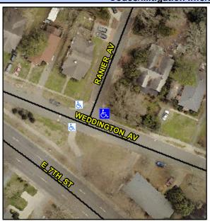
Street 1 Name Stop Condition-Street 2 Street 2 Name Stop Condition-Street 1 **WEDDINGTON AV** StopSign **RANIER AV** StopSign Possible Solutions: Remove & Replace Curb Ramp With Two New Directional Ramps or Equivalent. Surveyor Notes: N/A PROW/ADA: Not Found, R304.5.1, R304.2.2, R304.5.3
