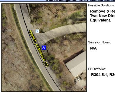
Stop Condition-Street 2 Street 2 Name Stop Condition-Street 1 **ENTRANCE** StopSign Remove & Replace Curb Ramp With Two New Directional Ramps or Equivalent.
