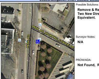
Street 1 Name Stop Condition-Street 1 Street 2 Name Stop Condition-Street 2 Remove & Replace Curb Ramp With **Two New Directional Ramps or** Equivalent.
