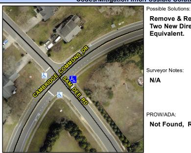
**SAM DEE RD** Street 1 Name StopSign Stop Condition-Street 1 Street 2 Name N/A Stop Condition-Street 2 N/A Remove & Replace Curb Ramp With **Two New Directional Ramps or** Equivalent.
