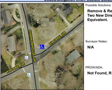
**SHANNONHOUSE DR** Street 1 Name Stop Condition-Street 1 StopSign Street 2 Name N/A Stop Condition-Street 2 N/A **Remove & Replace Curb Ramp With Two New Directional Ramps or** Equivalent.
