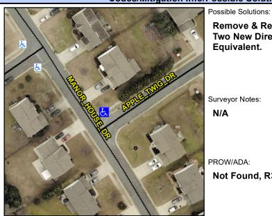
MANOR HOUSE DR Street 1 Name Stop Condition-Street 1 None Street 2 Name N/A Stop Condition-Street 2 N/A Remove & Replace Curb Ramp With **Two New Directional Ramps or** Equivalent.
