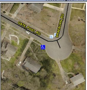
**GATE POST RD** Street 1 Name Stop Condition-Street 2 None Street 2 Name N/A Stop Condition-Street 1 N/A Possible Solutions: Remove & Replace Entire Ramp. Surveyor Notes: N/A PROW/ADA: Not Found, R304.2.2, R304.5.3
