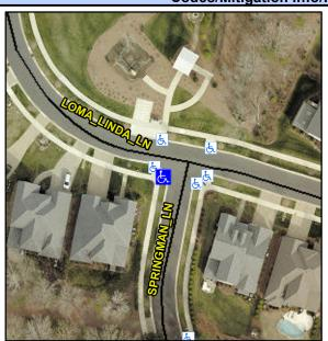
**SPRINGMAN LN** Street 1 Name Stop Condition-Street 1 StopSign Street 2 Name N/A Stop Condition-Street 2 N/A Possible Solutions: Remove & Replace Curb Ramp With Two New Directional Ramps or Equivalent. Surveyor Notes: N/A PROW/ADA: Not Found, R304.5.1, R304.5.3
