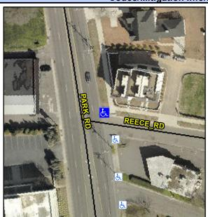
PARK RD Street 1 Name Stop Condition-Street 2 None Street 2 Name **REECE RD** Stop Condition-Street 1 StopSign Possible Solutions: Remove & Replace Curb Ramp With **Two New Directional Ramps or** Equivalent. Surveyor Notes: N/A PROW/ADA: Not Found, R304.5.1, R304.5.3
