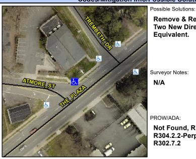
Street 1 Name Stop Condition-Street 2 Street 2 Name Stop Condition-Street 1 ATMORE ST StopSign **THE PLAZA** None Remove & Replace Curb Ramp With **Two New Directional Ramps or** Equivalent.
