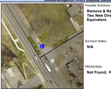
**AUDREY ST** Street 1 Name Stop Condition-Street 1 StopSign Street 2 Name N/A Stop Condition-Street 2 N/A **Remove & Replace Curb Ramp With Two New Directional Ramps or** Equivalent.
