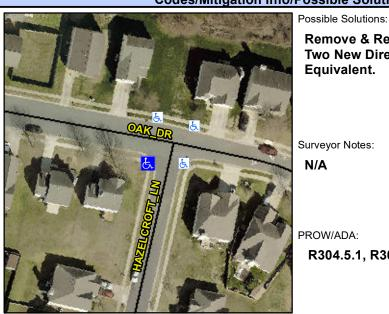
**HAZELCROFT LI** Street 1 Name Stop Condition-Street 2 StopSign Street 2 Name OAK DI Stop Condition-Street 1 None Remove & Replace Curb Ramp With Two New Directional Ramps or Equivalent.
