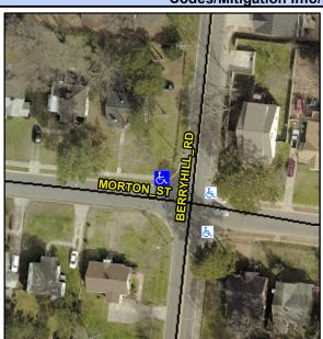
**BERRYHILL RD** Street 1 Name Stop Condition-Street 1 None Street 2 Name N/A Stop Condition-Street 2 N/A Possible Solutions: Remove & Replace Curb Ramp With Two New Directional Ramps or Equivalent. Surveyor Notes: N/A PROW/ADA: Not Found, R304.5.1
