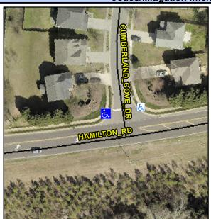
**CUMBERLAND COVE DR** Street 1 Name Stop Condition-Street 2 None **HAMILTON RD** Street 2 Name Stop Condition-Street 1 StopSign Possible Solutions: Remove & Replace Curb Ramp With Two New Directional Ramps or Equivalent. Surveyor Notes: N/A PROW/ADA: R304.5.1
