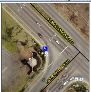
**E INDEPENDENCE BV** Street 1 Name Stop Condition-Street 2 Signal Street 2 Name N/A Stop Condition-Street 1 N/A Possible Solutions: Remove & Replace Entire Ramp. Surveyor Notes: N/A PROW/ADA: Not Found, R304.5.1, R304.5.3
