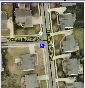
**BECKET RIDGE RD** Street 1 Name Stop Condition-Street 2 None DONNEGAL FARM RD Street 2 Name Stop Condition-Street 1 StopSign Possible Solutions: Remove & Replace Curb Ramp With Two New Directional Ramps or Equivalent. Surveyor Notes: N/A PROW/ADA: Not Found, R304.5.1
