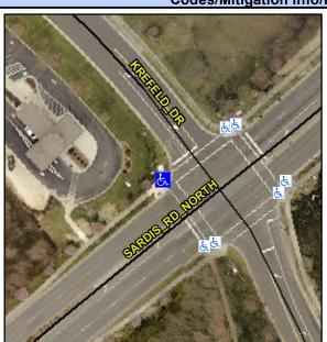
**CROWNPOINT EXECUTIVE DR** Street 1 Name Stop Condition-Street 2 Signal Street 2 Name **KREFELD DR** Stop Condition-Street 1 Signal Possible Solutions: Remove & Replace Curb Ramp With Two New Directional Ramps or Equivalent. Surveyor Notes:
