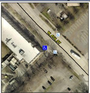
Street 1 Name Stop Condition-Street 1 Street 2 Name Stop Condition-Street 2 **ENTRANCE** StopSign W 4TH ST None Possible Solutions: Remove & Replace Curb Ramp With **Two New Directional Ramps or** Equivalent. Surveyor Notes: N/A PROW/ADA: Not Found, R304.5.3
