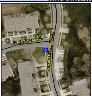
SUMMERFIELD RIDGE LN Street 1 Name Stop Condition-Street 2 Street 2 Name LITTLE STREAM CT Stop Condition-Street 1 StopSign Possible Solutions: Remove & Replace Curb Ramp With **Two New Directional Ramps or** Equivalent. Surveyor Notes: N/A PROW/ADA: R304.2.2, R304.5.3
