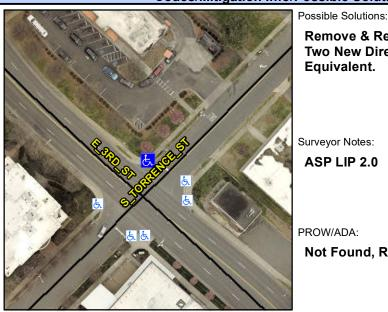
Street 1 Name Stop Condition-Street 1 Street 2 Name Stop Condition-Street 2 Remove & Replace Curb Ramp With Two New Directional Ramps or Equivalent.
