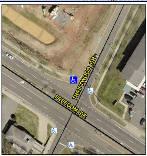
THRIFTWOOD DR Street 1 Name StopSign Stop Condition-Street 1 Street 2 Name N/A Stop Condition-Street 2 N/A **Remove & Replace Curb Ramp With Two New Directional Ramps or** Equivalent.
